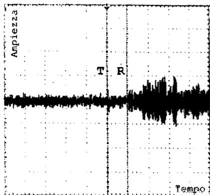
Figure 3: Transmission measures at 100 KHz in region B (medium level flaw)
