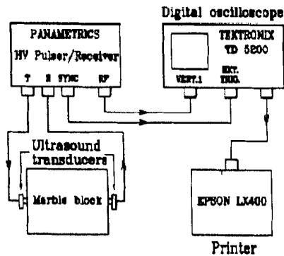
Figure 1: Measurement equipment used in in-field testing
