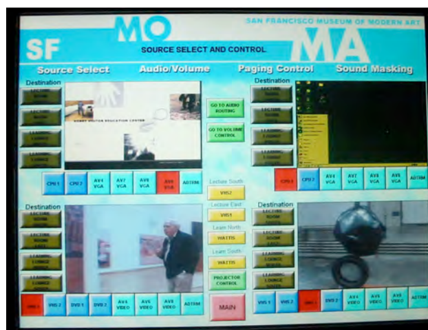
Fig. 3: Front desk control console interface: Source Selection screen for the four data projectors
