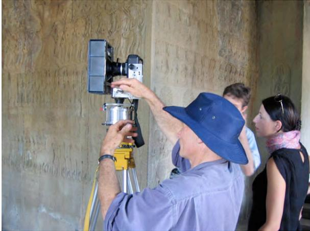
**Fig 4:** Digital SLR camera mounted on a tripod, with ‘hood’ on the ultra wide angle lens. Northeast corner pavilion Angkor Wat, Angkor, Cambodia, 2004.
