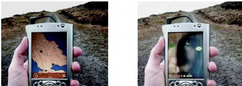
Fig. 2: Our prototype: map interface(left) is default; when story arrives, a character's face appears (right)
