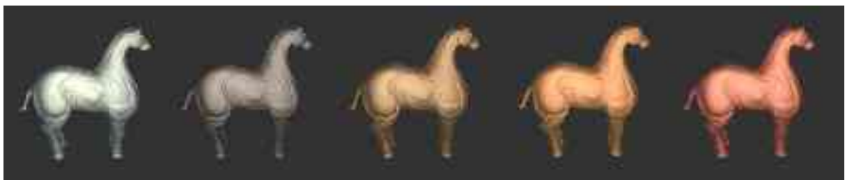
Fig 15: Three simulated replicas in bronzes between the fundamental compounds of pure Tin (left) and pure Copper (right)
