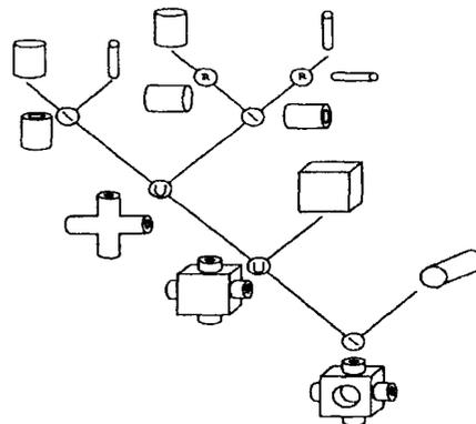
**Figure 3: Example of a CSG tree. Operations: R (rotation),  $\setminus$  (subtraction), U (union).**
